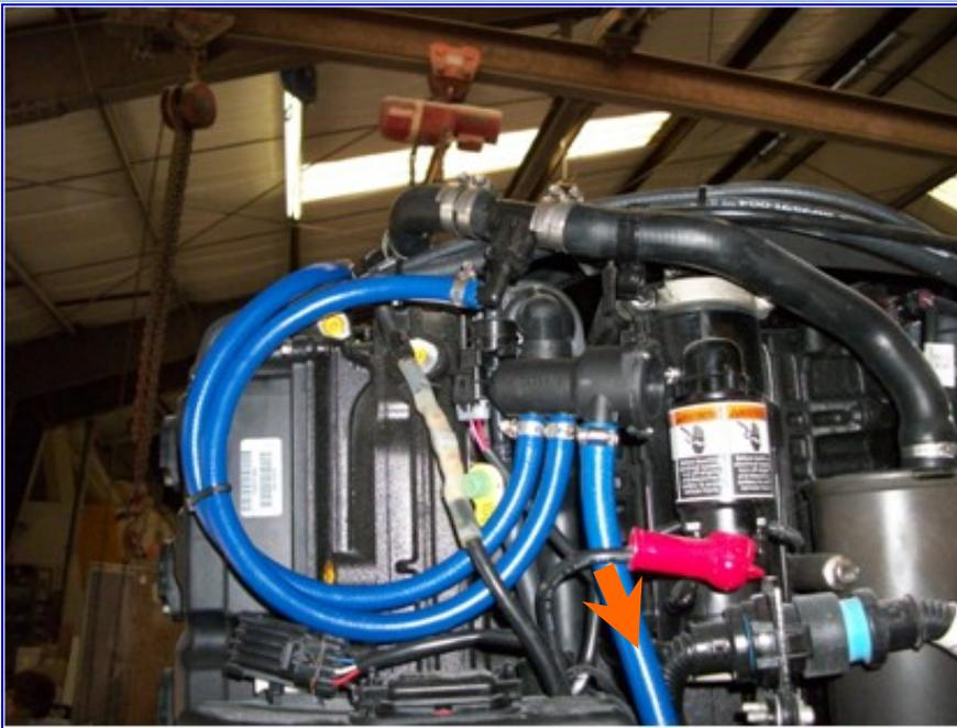
Step 5: Mount the SF 200 unit with black cable ties provided as shown in picture to the Left. Route the flush injector lines to injectors # 1 & # 2 as shown. Using stainless steel clamps provided secure the lines. Attach the 1/2” main feed line to the inlet as shown.
