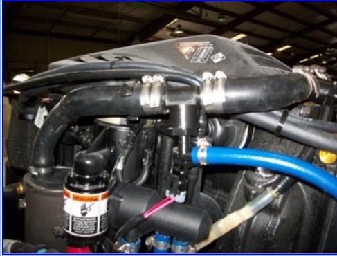
Step 4: Insert the Verdao Easy Injector # 2 in this location and “double” clamp as shown in the picture to the left. Using the clamps provided install the 3/8” injector line as shown.
