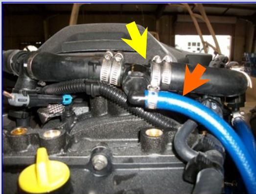
Step 2: Insert the Verdao Easy Injector # 1 in this location and "double" clamp as shown in the picture to the left. Using the clamps provided install the 3/8" injector line as shown by the orange arrow.
